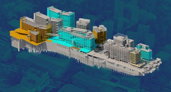
The structure and environment of the project are integrated such that the overall carbon footprint (embodied and operational) is optimized. Extensive adoption of precast construction was deployed in the design for all structural elements to facilitate off-site fabrication, reduce time of construction and limit site activities. Promotion of sophisticated design techniques have also helped lower cost as well as environmental impact of the building structure.
